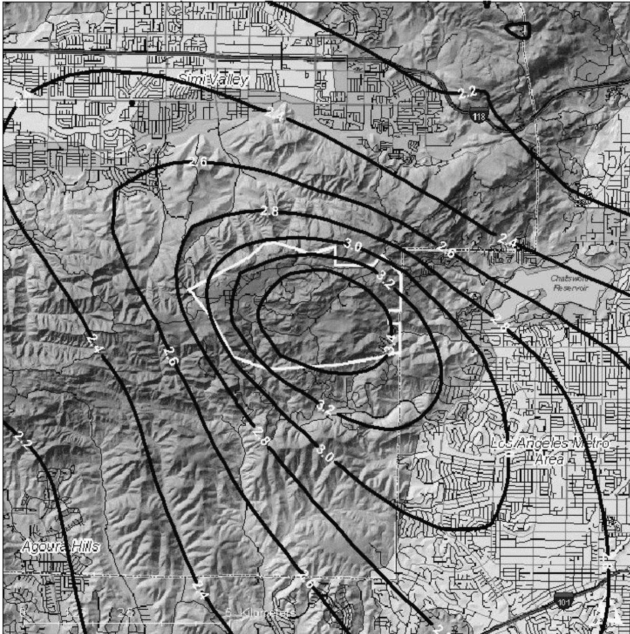
**Figure 3-11.** Average Concentration Pattern for all RET Point Sources Using the Uniform Diurnal Emissions Profile
