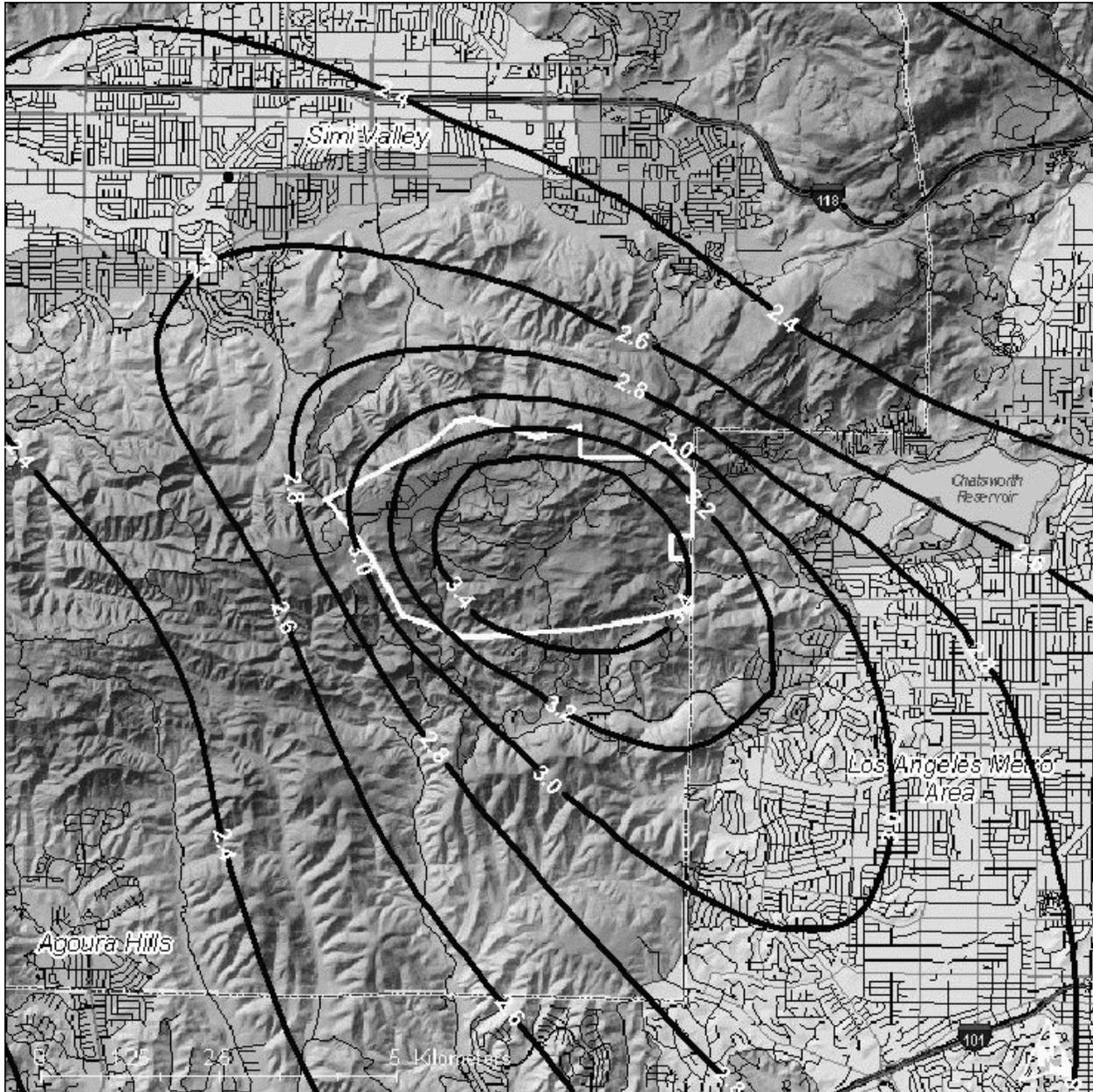
**Figure 3-13.** Average Concentration Pattern for all RET Area Sources Using the Uniform Diurnal Emissions Profile
