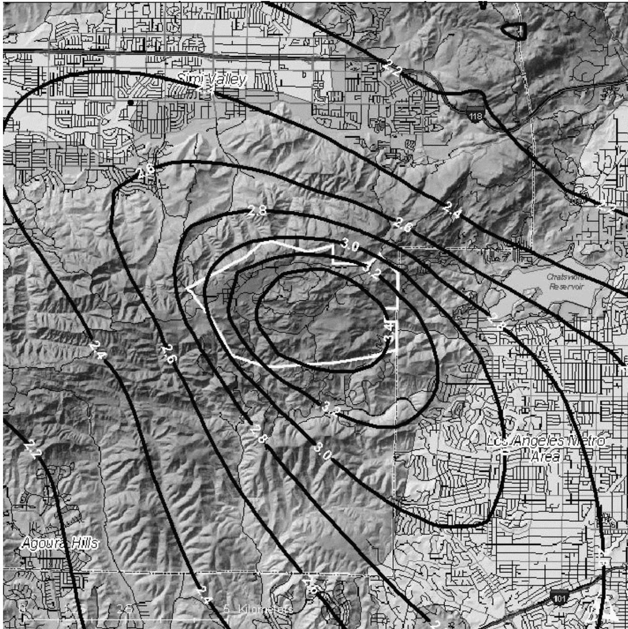
**Figure 3-12.** Average Concentration Pattern for all RET Area Sources Using the Best-Estimate Diurnal Emissions Profile
